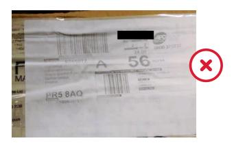
The print must be correctly positioned on the label, with white space around the barcode.
